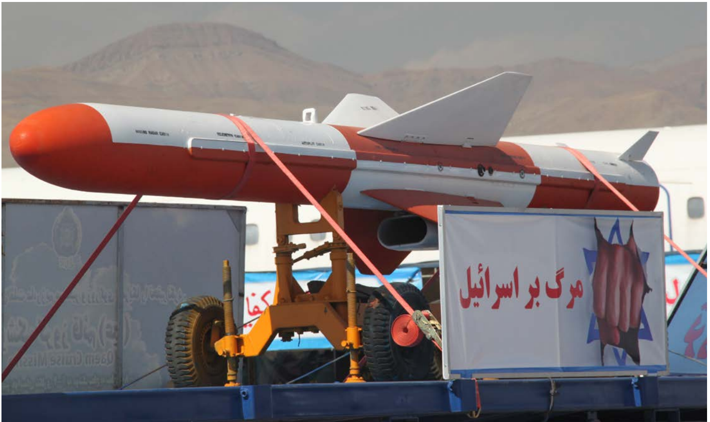
Photo above: Iranian defense industries have produced a range of anti-ship cruise missiles based on Chinese models, including this air-launched version of the C-802 Noor missile with a range of between 75 and 120 kilometers. Credit: The author's collection.
