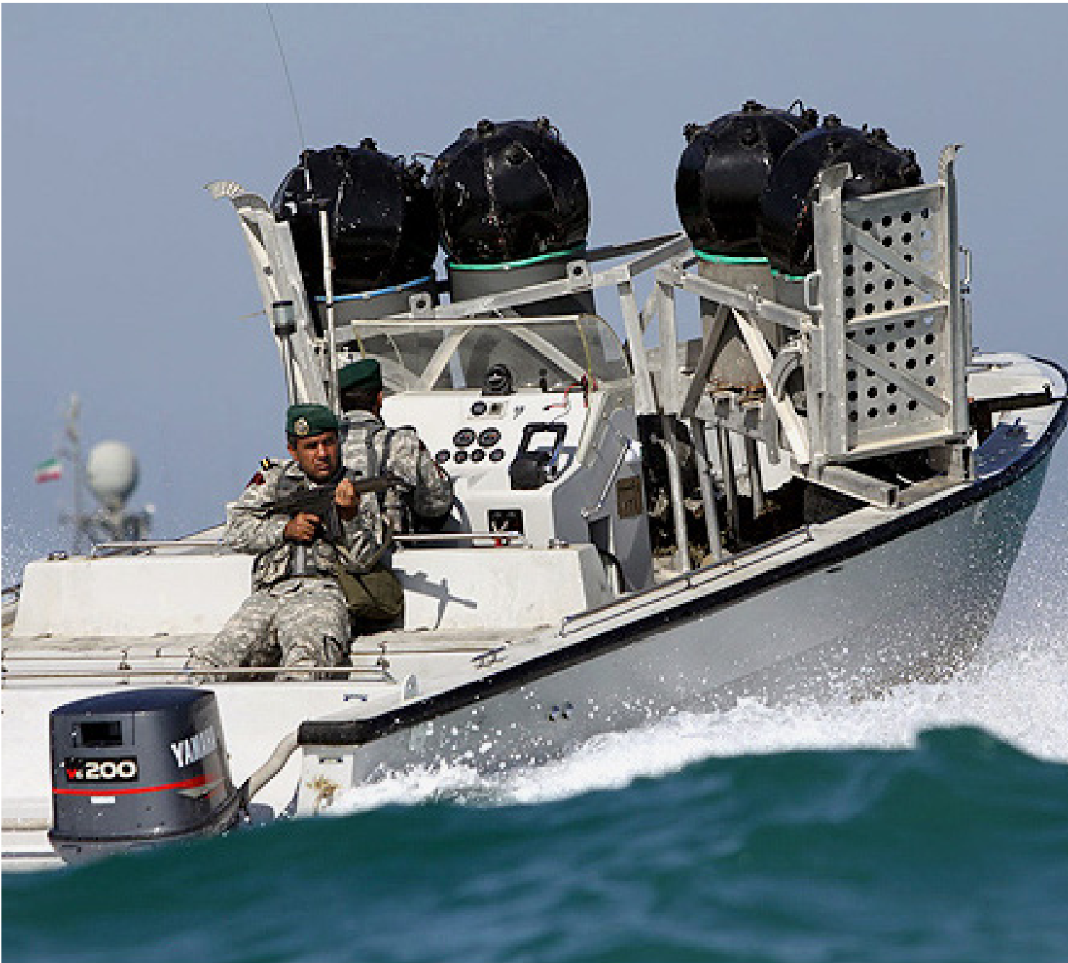
Photo above: Both the Iranian national and revolutionary navies regularly practice mining the Gulf waters. Here an IRIN speedboat is rigged to rapidly dispense four floating mines, two from each side. IRGCN boats usually carry two mines. Credit: FarsNews.
