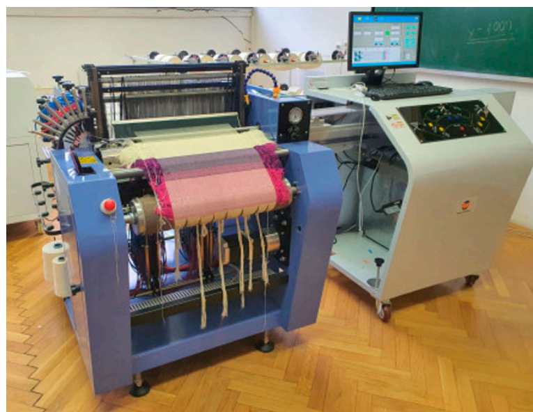
Figure 1. Laboratory weaving machine—Fanyuan instrument/model DW598/Hafei Fanyuan instrument, Hefei City, China.
