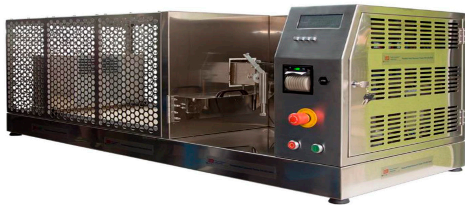
Figure 8. Laboratory test equipment for determining the resistance to radiant heat according to the method EN ISO 6942 [21].
