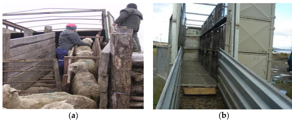
Figure 3. (a) Loading sheep using a wooden ramp; (b) truck with metallic adjustable pens and double flooring, also showing the metallic loading ramp.
