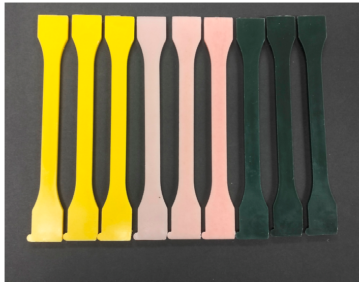
Figure 4. Visual aspect of the injected PLA specimens with 2, 4 and 6 wt% of natural pigment-based MBs developed.
