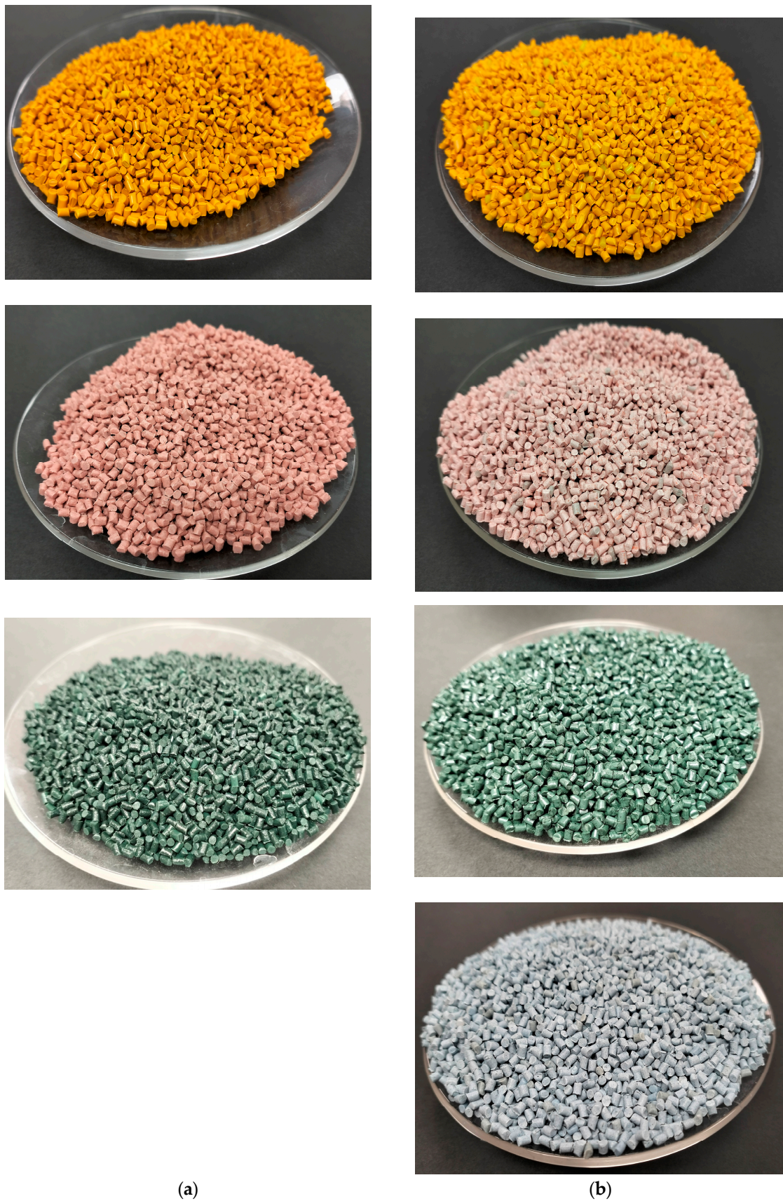
Figure 2. Natural pigment-based MBs developed (a) based on PLA matrix, (b) based on PBS matrix.
