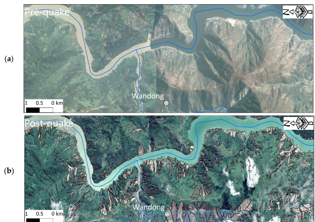
Figure 3. Map showing the coseismic landslides based on pre- and post-quake Google Earth images located in the Wangdong area. (a) Pre-quake satellite image. (b) Post-quake satellite image.
