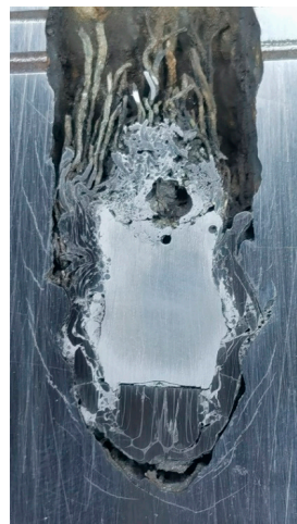
Figure 8. Bending and backflow fracture mode of tungsten fibers during penetration of WF/Zr-MG rod [20].
