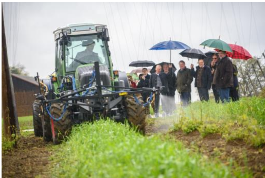
Fig. 5.4: Demonstration of sensor-controlled plant protection equipment treating rows of hops
