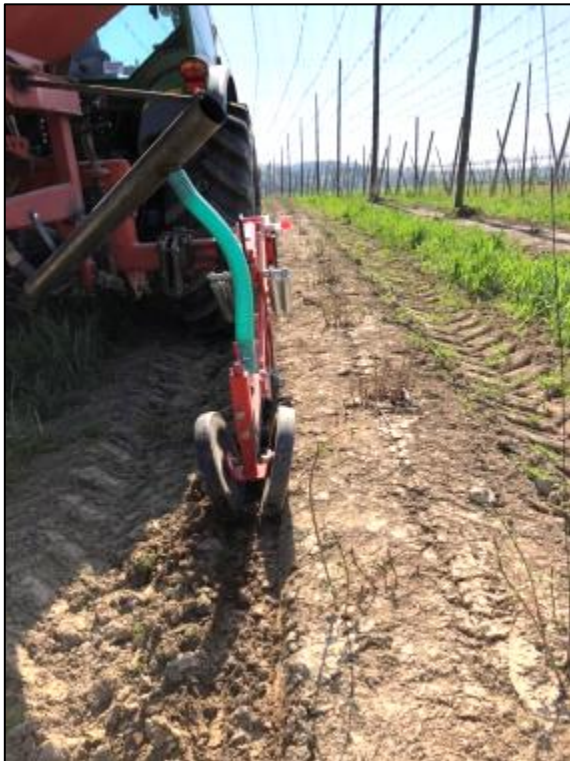
Fig. 1.11: Depositing the fertilizer depot beside the row of hops
