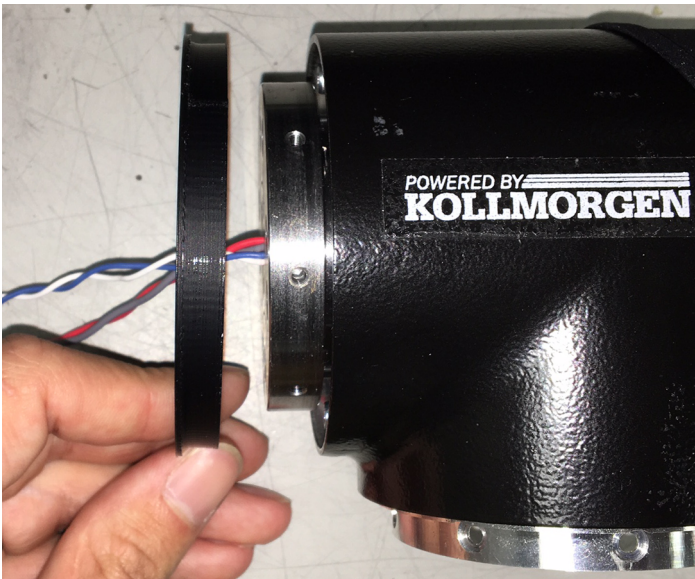
Figure 4: Placing the plastic ring into the housing pilot.
