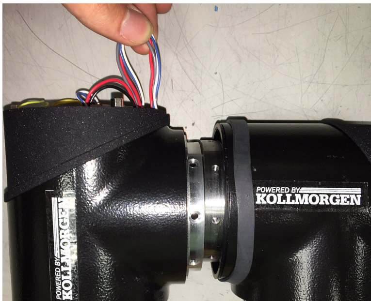
Figure 10: Keep wires tight to avoid pinching
