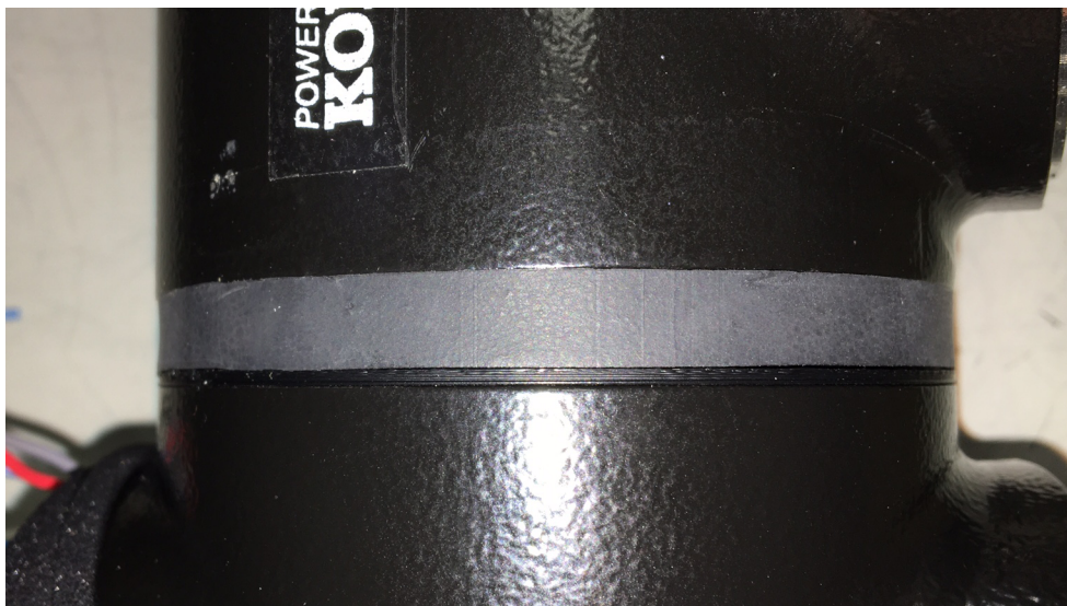
Figure 7: Move the flexible seal band so it holds the plastic ring in place.
