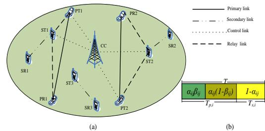
Fig. 1. Cooperative cognitive radio networks (a) system architecture (b) time duration division.
