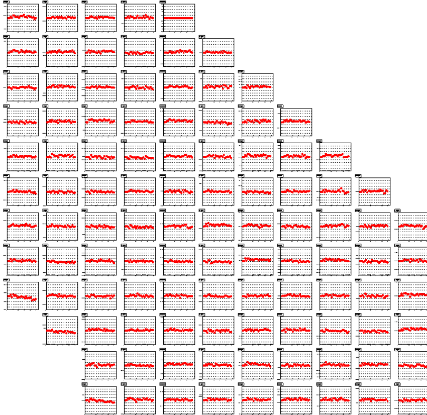
FIG. 5: Gain variations for each IC crystal in the upper right quadrant, as a function of time over the whole run, as measured by the laser monitoring system. Dashed horizontal lines are separated by 5%.
