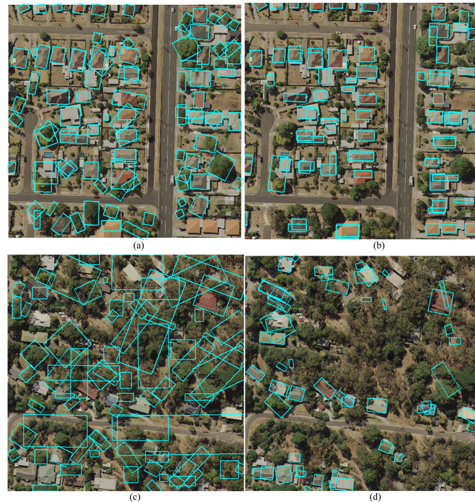
Figure 7: Building detection by the previous (left) and the improved (right) algorithms on two samples from Knox.
