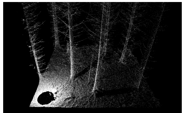
Figure 1. Example of a point cloud from a laser scanned forest plot. Shading occur behind the trees and under the measuring instrument. The number of shaded areas can be reduced if several instrument positions are used.
