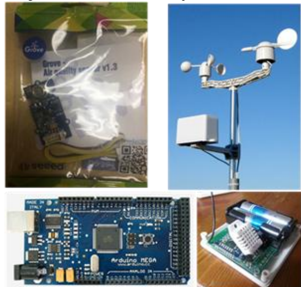
Figure 9: Sensors used: from left to top air quality sensor, weather station, Arduino system, humidity and temperature.
