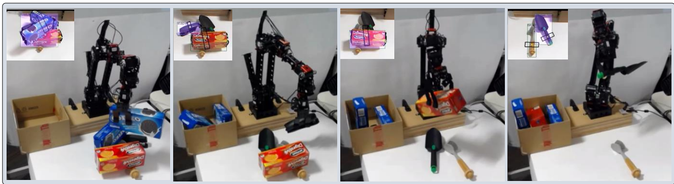
Figure 5: Real-world robotic grasping setup. An image acquired from Kinect is fed to Faster-RCNN [Ren et al. , 2015] to generate object proposals. These are fed to the proposed GraspNet to generate grasp inferences which are used by a robotic arm for robotic grasping. Both Faster-RCNN and GraspNet run on Nvidia Jetson X1 (see the video at: https://youtu.be/byEmAOImC90 ).
