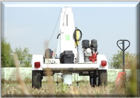
ESS1000 WITH 950-1000 Pound hammer (seismic energy source)
