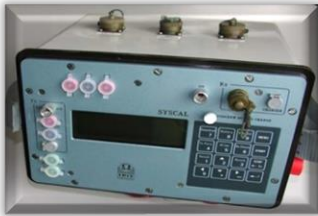
SYSCAL Junior R1 Plus Switch-72 Resistivity meter, SYSCAL Junior R1 Plus Switch, Iris Instrument, France
