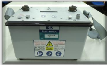
SYSCAL SWITCH Pro-48 Resistivity meter (EXTENSION UNIT), SWITCH Pro 48, Iris Instrument, France
