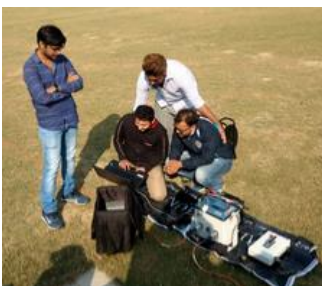
Multi-electrode Restivity Meter (with 120 electrodes), Syscal R1 plus by Iris Instruments, France
