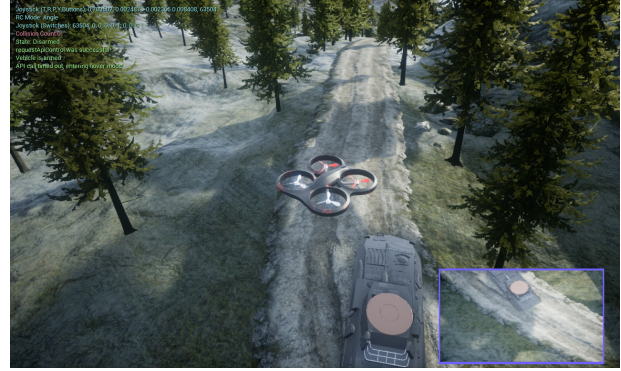
Figure 1: Screenshot of AirSim environment and landing task. Inset image in lower right corner: downward-facing camera view used for extracting the position and radius of the landing pad, which is part of the state space.
