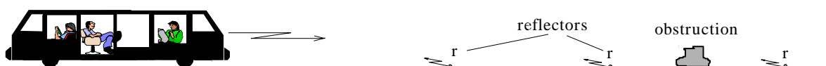
Fig. 1. Proposed arrangement of reflectors along a railway for obstruction detection within the line-of-sight region using microwave radar sight region a microwave radar is used, and for the
