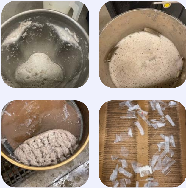
Upper left: Waring blender Upper right: British disintegrator (deflaking) Bottom left: Screening (accepts) Bottom right: Screening (rejected material)
