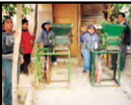
Pedal power is used for husking coffee beans at As Green As It Gets, an economic development organization.
