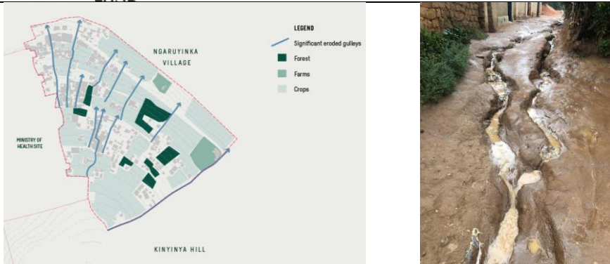
Figure 1: Ngaruyinka Village – existing location of significant eroded gullies and picture of uncontrolled stormwater channels in the community
