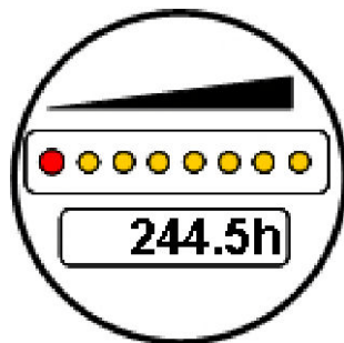
Fig. 6-20 Battery charge indicator with 7 yellow LEDs, red LED to the left of yellow LEDs
