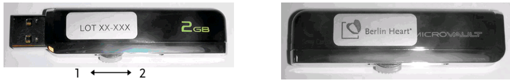
Fig. 15-6 Left: USB stick with extended plug (operating position); Right: USB- stick with retracted plug (position to transport and store the stick)
