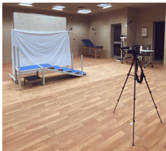
Figure 1. The experimental setup, which includes a staircase, a camera mounted on a tripod, a weight beam eye-level scale, a measurement bed, a start mark on the floor, and an end mark on the fifth step.
