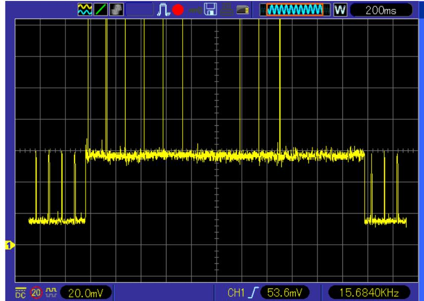
Figure 4-1. Active SSID Scanning with Modem-sleep Mode Enabled (X: 200 ms/div, Y: 20 mA/div)
