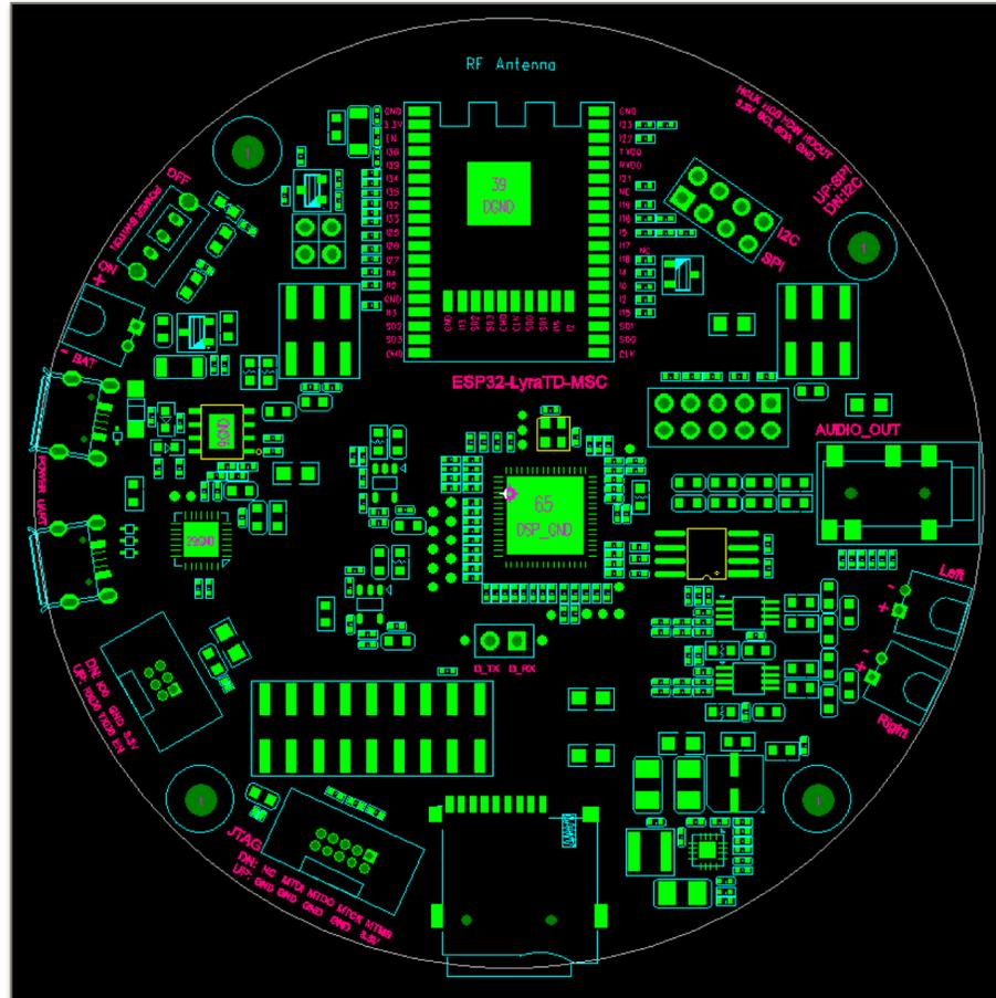
Figure 2-5. Reference Design for Module Placement
