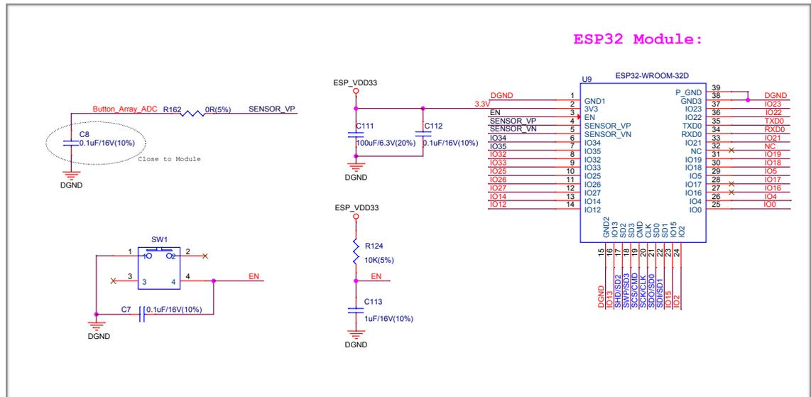
Figure 1-6. Reference Circuit for Part of ESP32 Pin Configuration
