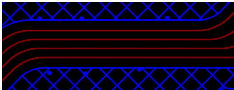
Figure 2-16. Reference Design for TouchPad Traces Routing
