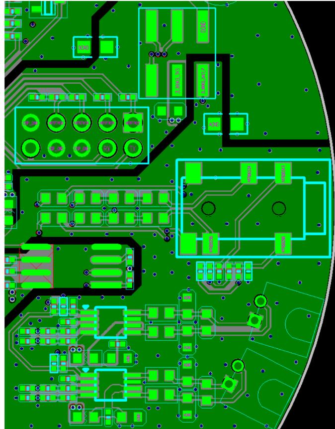
Figure 2-11. Reference Design for Ground Trace Routing
