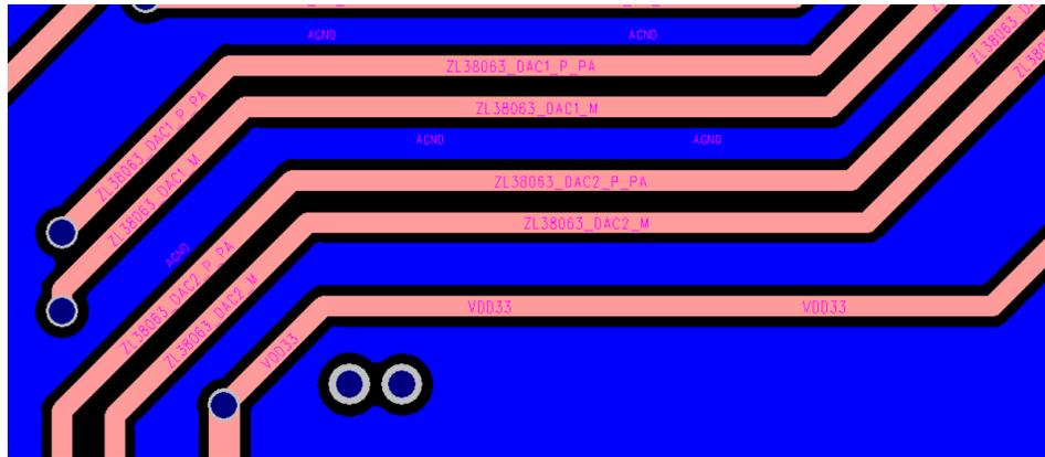
Figure 2-15. Reference Design for Audio Signal Trace Routing
