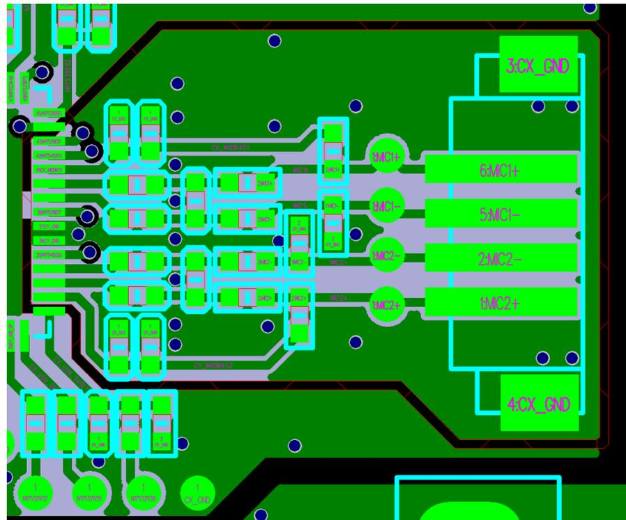
Figure 2-11. Reference Design for Ground Trace Routing
