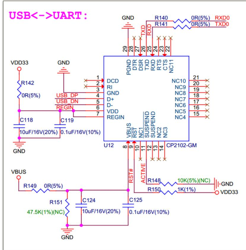
Figure 1-7. Reference Circuit for USB-UART Chip
