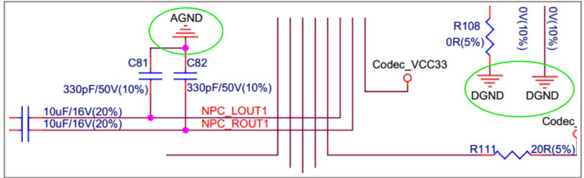
Figure 1-5. Reference Circuit Design for a Codec Ground Plane
