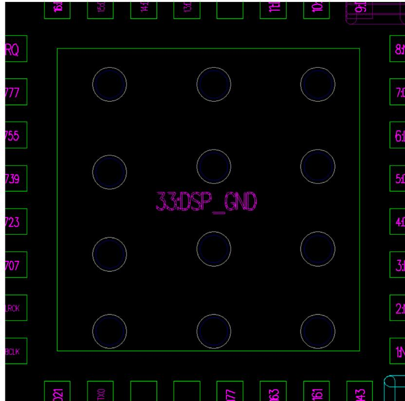
Figure 2-11. Reference Design for Ground Trace Routing
