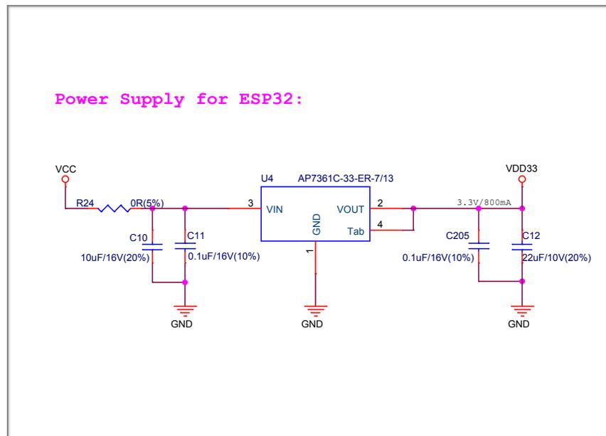
Figure 1-2. Power Supply Management Circuit for Peripherals
