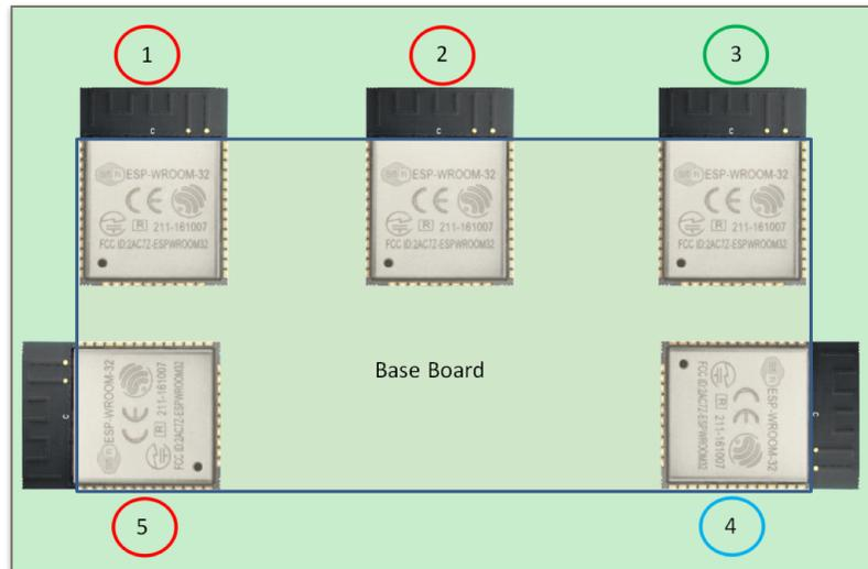
Figure 2-3. ESP32 Module Antenna Position on Baseboard
