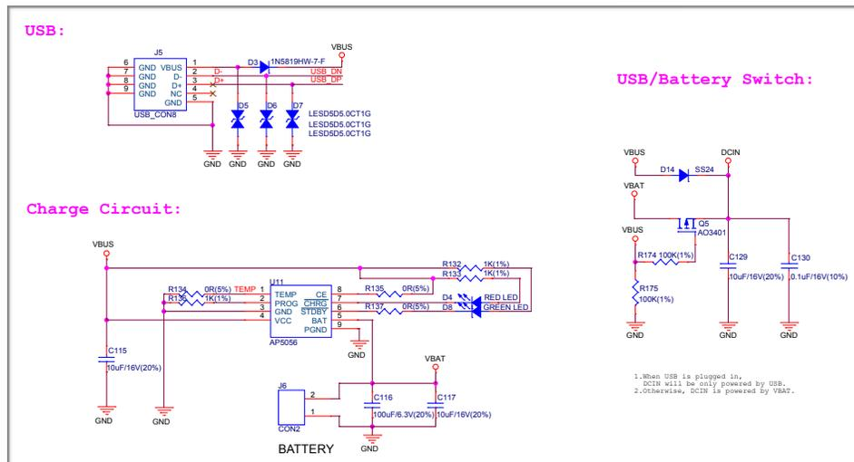
Figure 1-1. USB/Battery Power Supply Circuit
