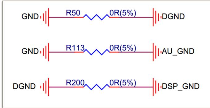
Figure 1-3. Circuit for Splitting Ground Planes
