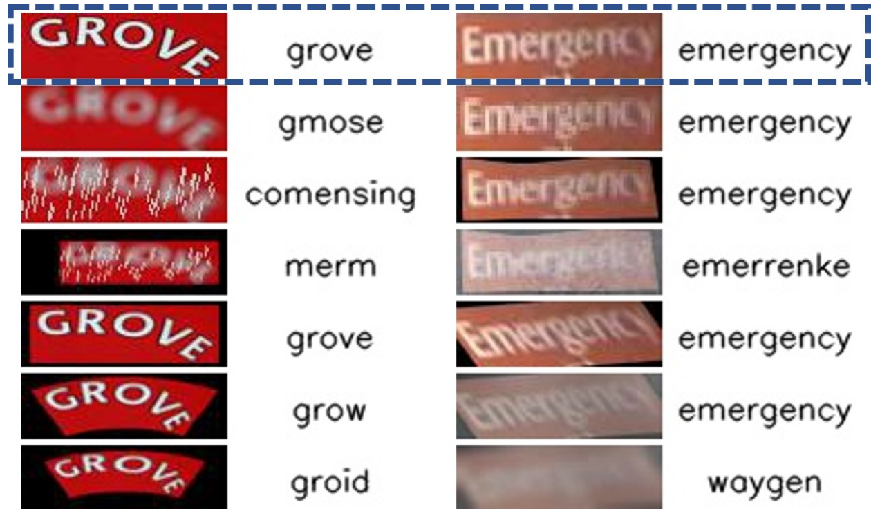
Figure 5.1: Typical errors in scene text recognition caused by image transformations. Row 1: two original text images with their text labels. Row 2-7: the augmented text images with different image transformations. Column 2, Column 4: text recognition results for images in column 1 and 3 respectively .
