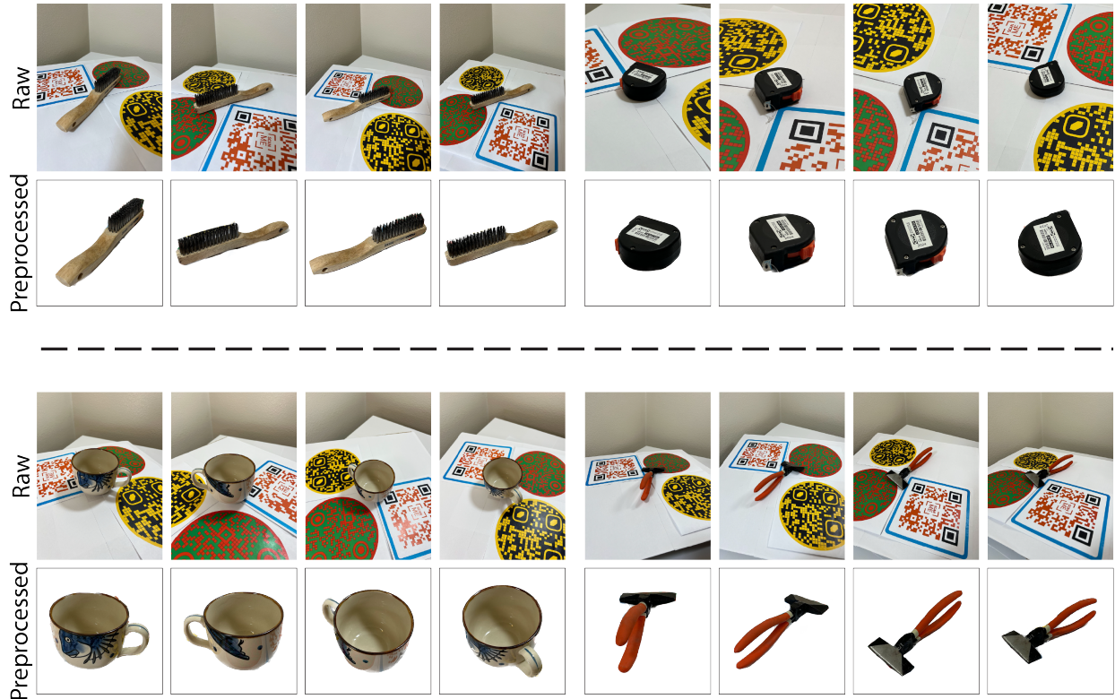
Figure 5.4: Visualization of raw and preprocessed multi-view images. Raw images represent the images directly output from the capture device, i.e., iPhone 13 Pro. We process raw images with segmentation and cropping before feeding them into the models.
