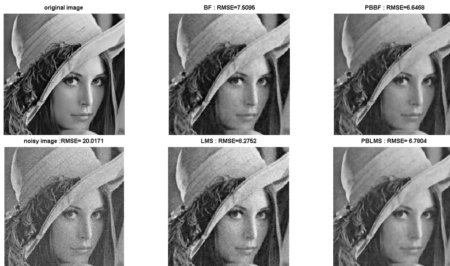
Fig. 1: Example of the Lena image. Top row, left: original image, middle: bilateral filtering, right: patch-based bilateral filtering. Bottom row, left: noisy image, middle: local M-smoother, right: patch-based local M-smoother.
