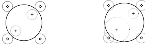
Figure 2: Position of the decision hypersphere can be influenced by confidence. Left picture shows the position of decision hypersphere (black circle) for uniformly distributed confidences (grey circles). After increasing of confidence for left bottom point, the decision circle is moved in such a way, that the affected point is placed further inside.
