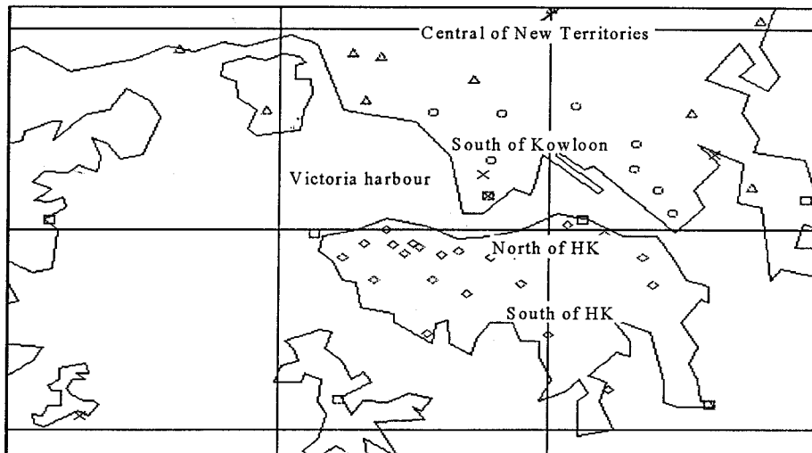
Fig. 2. Rain gauges distribution and layout of Hong Kong
