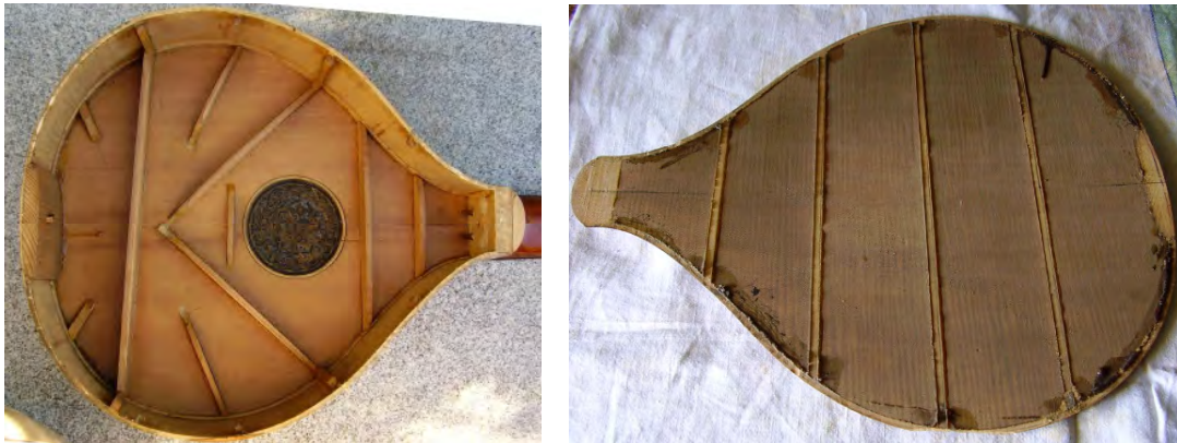
Figure 6.27: Left: The distinctive soundboard bracing, with two diagonal bars forming a characteristic 'V' shape below the rose, on a guittar by Preston, private collection, UK. Right: The bracing of the back consisting of four horizontal bars, which have been removed during restoration (photos by A. Robb, < http://www.art-robb.co.uk/EG.html >, accessed 27/11/10).
