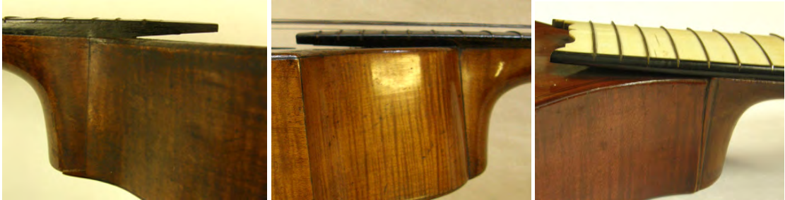
Figure 6.50: Details of the ‘floating’ fingerboard end on three examined guitars. Left to right: Liessem, EUC [1070]; Hintz, DCK [MI/A10]; unsigned, EUC [1592].
