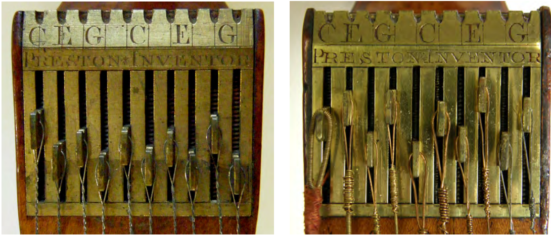
Figure 7.28: Two identical watch-key machines by Preston bearing engravings of the common guittar tuning in C and the words 'PRESTON*INVENTOR' below. Left: Ashmolean Museum, Oxford, [D.1:1]. Right: Museum für Musikinstrumente der Universität, Leipzig, [5005].
