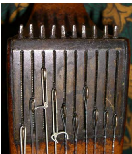
Figure 7.20: Detail of the watch-key machine for ten strings on a bowl-back guittar by Hoffmann dated 1758. T. Takeuchi collection, London (< http://www.vihuelademano.com/current/pages/guittar-hoffmann1758.htm >, accessed 27/4/2009).
