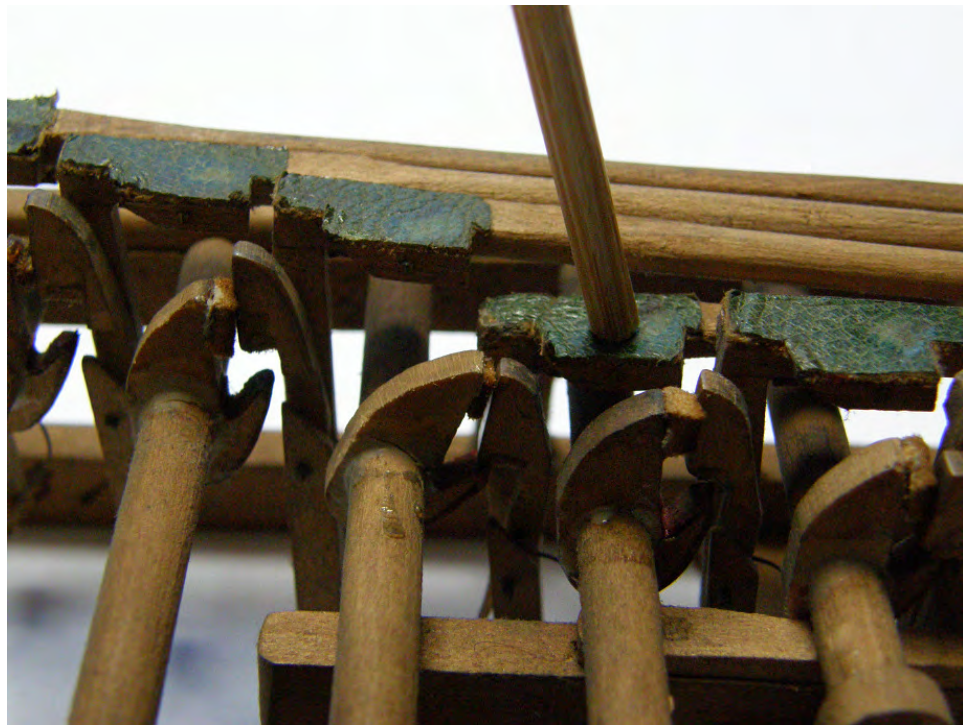
Figure 7.104: Top: The removable internal piano-key mechanism of GNN [MIR 857]. Bottom: Detail showing the escapement action using a claw and cam system on the piano-key mechanism of GNN [MIR 857]. When the piano key (in this case simulated with a wooden stick) is depressed, the hammer is forced to strike the string and immediately returns back to its original position by means of a wire spring.
