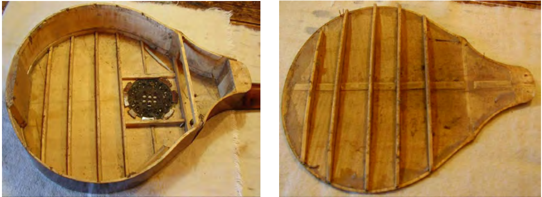
Figure 6.21: Horizontal bracing comprising six bars on the soundboard and six bars on the back, on a bell J-top guitar by Gibson (photo by A. Robb, < http://www.art-robb.co.uk/EG.html >, accessed 27/11/10).
