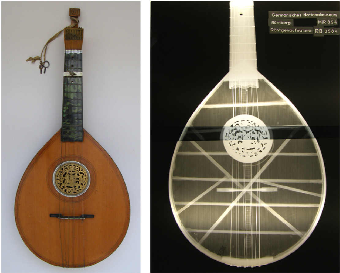
Figure 6.32: Left : Front view of an unsigned egg-shaped guitar, possibly by Longman & Broderip, Germanisches Nationalmuseum, Nuremberg, [MIR 854]. Right : X-ray photograph of GNN [MIR 854] showing the interior bracing of the soundboard and back. The soundboard bracing consists of a horizontal bar above rose towards neck and two long diagonal bars placed at an 'X'-shape intersecting under the bridge, with two asymmetrical diagonal bars placed on the bass and treble sides. The bracing of the back consists of six horizontal bars. A number of short and thin rectangular bars, with their wood grain perpendicular to the strings, have been used along on the middle joint on the back for extra support.
