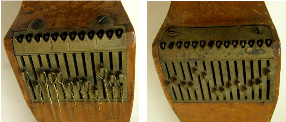
Figure 7.13: The watch-key machines on two keyed guitars by Longman & Broderip in the Museum für Musikinstrumente der Universität Leipzig, Leipzig, [628] (left) and [627] (right). Note that both machines have been attached on the head with two screws in order to withstand the tension of the twelve strings and to prevent distortion of the machine.
