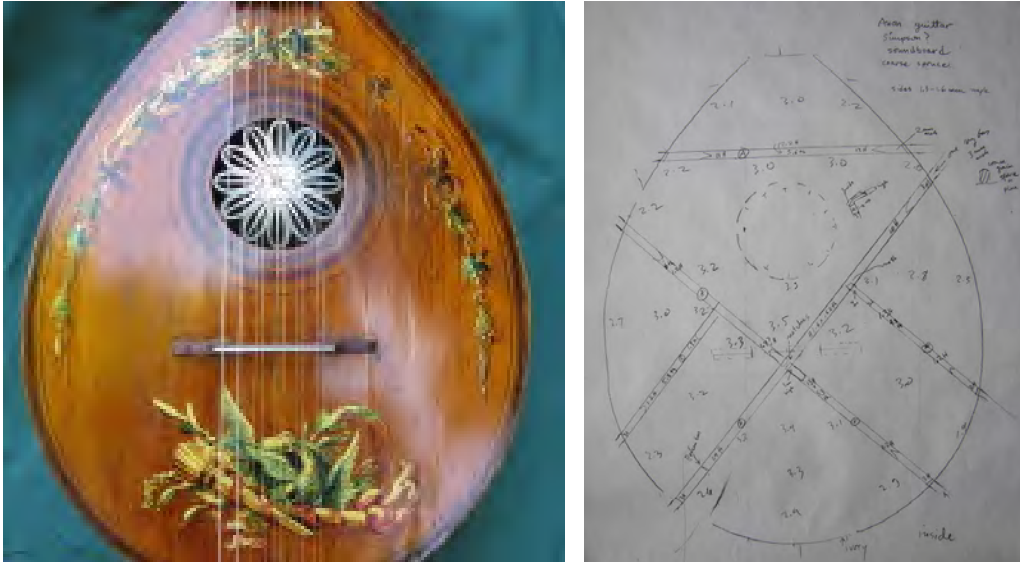
Figure 6.33: Left: Front view of an unsigned egg-shaped guittar. A. Rutherford collection, New York. The painted decoration on the soundboard may be a later addition. Right: Technical drawing showing the horizontal and 'X'-shaped bracing on the soundboard of this instrument (photo and drawing courtesy of A. Rutherford).
