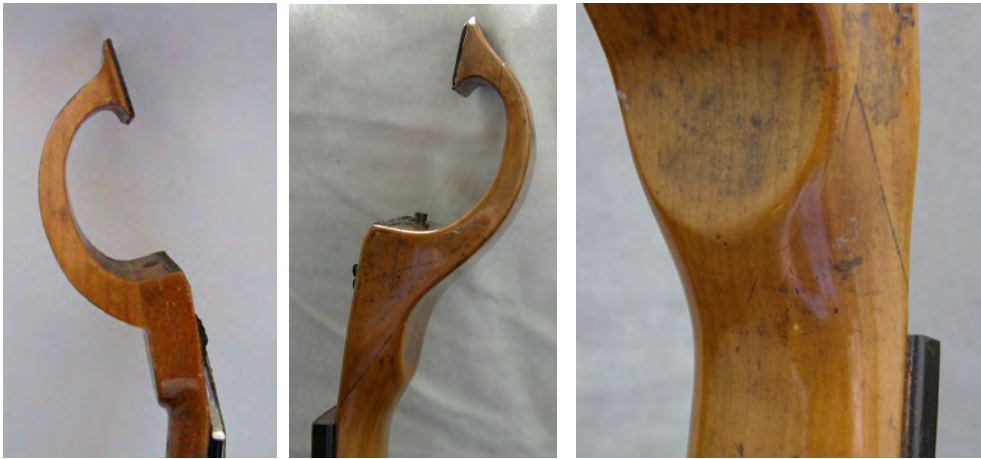
Figure 6.48: Details of the straight neck-head joint on a keyed guitar by Longman & Broderip, GNN [MIR857] ( left ), and of the pointed neck-head joint on a keyed guitar by Claus, BCP [8051] ( middle and right ).
