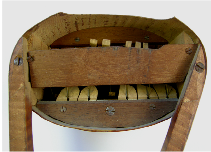
Figure 7.141: The underside of Smith's Patent Box belonging to SMM [43-307]. Note that two of the seven hammers are missing.
