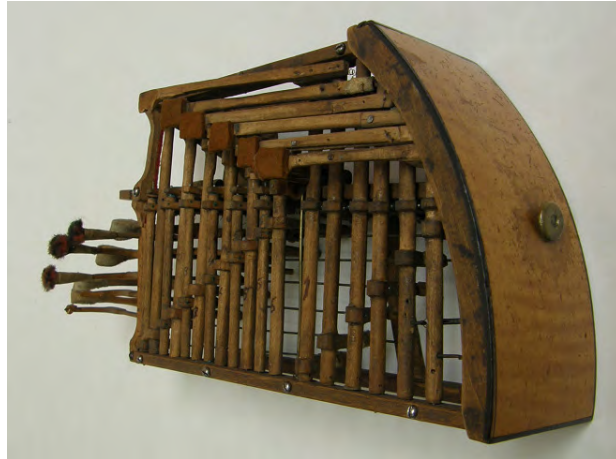
Figure 7.129: Detail of the 'hautboy' stop on the piano-key mechanism of MUL [628]. Note also the numbers 1 to 6 written in ink on the hammer levers.
