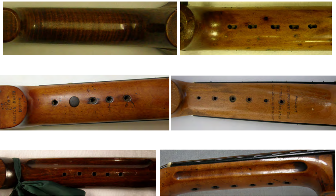
Figure 6.43: Examples of typical guittar necks. Left to right, top: Liessem EUC [1070], Hintz EUC [1066]. The neck and head on EUC [1070] are carved of a single piece of figured maple; the neck has no capotasto holes. Middle: Preston MUL [5005], Longman & Broderip GNN [MIR 857]. Note that on both instruments the fingerboard overlaps the neck at the sides. Bottom: Gibson EUC [309], Clagget HMH [MS129]. Note the distinctive groove carved along the bass side on both guittars.
