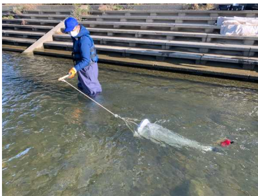
Photo 3-10. Stepping into the river and collecting samples
