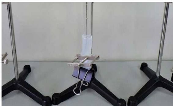
Photo 4-13. Securing of a tube tip
