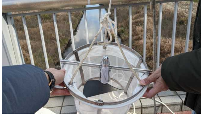
Photo 3-8. An example of fixation of plankton net
