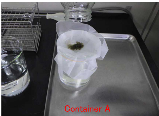
Photo 4-1. Filtration of impurities through a net
