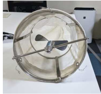
Photo 3-6 Case 2. An example of fixation of the flowmeter with a metal frame
