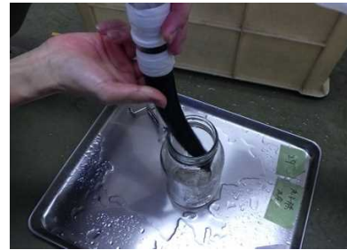
Photo 3-16. Transfer of samples from a bottom pipe to a container
