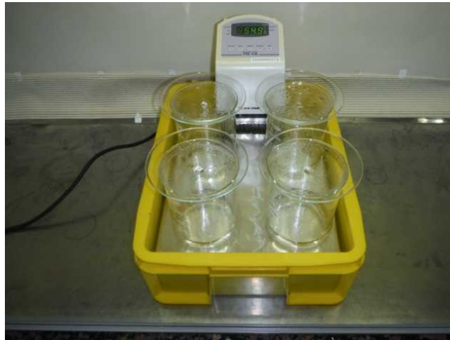
Photo 4-10. Warming of containers in a water bath
