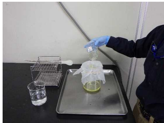
Photo 4-20. Filtration of water to collect samples
