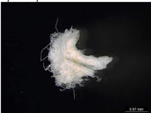
4. Foam (expanded): spherical and expanded pieces
