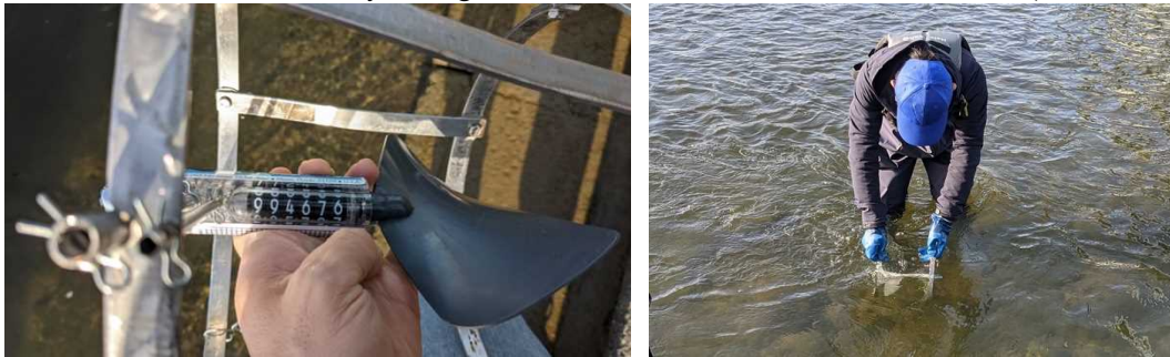
Photo 3-11. Measurement of flow velocity with flow meter
