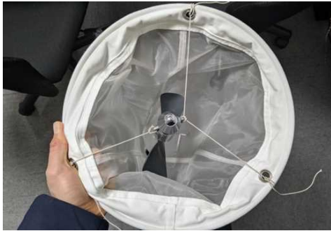
Photo 3-5 Case 1. An example of fixation of the flow meter with strings
