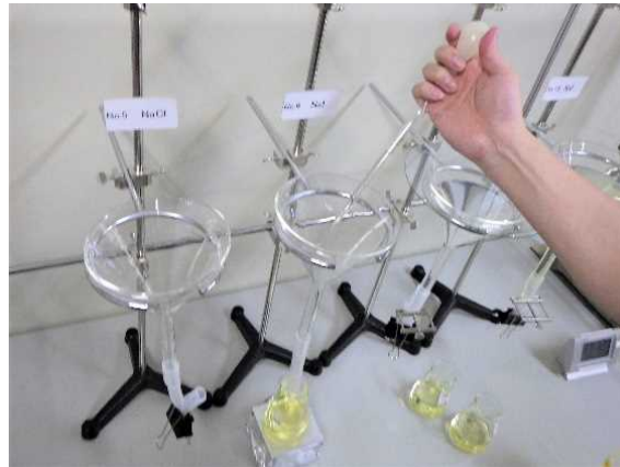
Photo 4-19. Rinsing out the remaining samples
