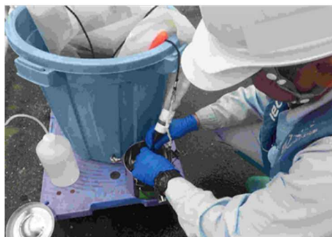
Transfer of samples from a cod end to a storage container
