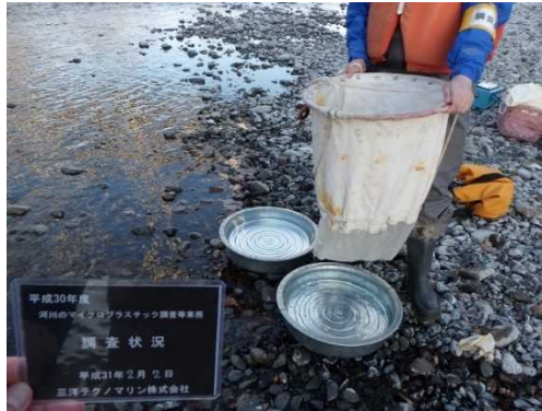
Filtration of river water with a net with 0.1 mm mesh openings
