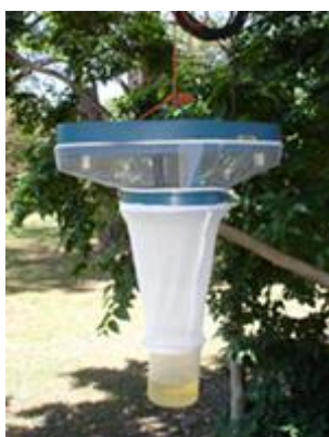
Figure 2. OVI light/suction trap, manufactured by Onderstepoort Veterinary Institute, South Africa
