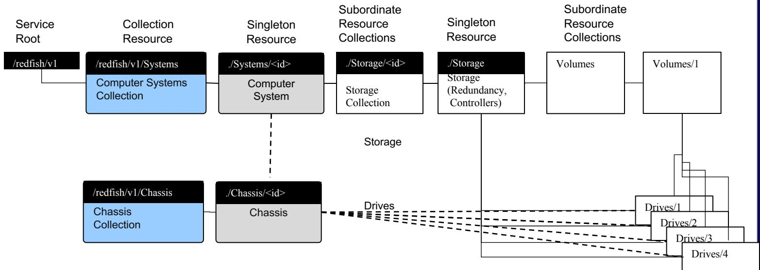
Note that the Volumes are in Collections off of the Storage resource, drives are in arrays off of the storage resource and optionally the Chassis.
