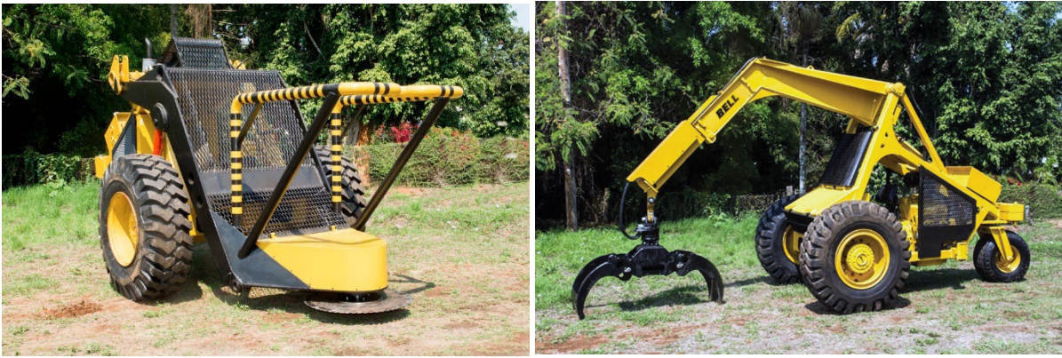
FIGURE 5.1. A) Custom-built cutting machine for clearing bush encroachment. B) Bell skid steer loader used to stack trees after cutting. Photo credit: http://bushclearingsolutions.co.za
