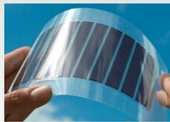
flexible encapsulation for solar cells
