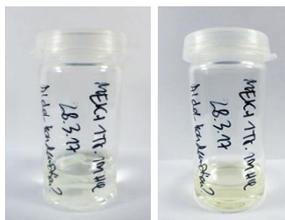
MEK treated with HCl, after 24 h (left) and after 7 d (right)
