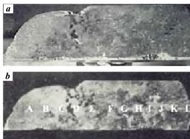
Figure 3. a , Heterogeneous etching of the Delhi pillar sample section using HCl as etchant, indicating non-uniform distribution of entrapped slag inclusions 11 . b , Polished section after etching in Stead's reagent 11 . Bright regions are those where P content is higher. Variation in P content and the relatively high percentage of P in the surface must be noted. Microstructures marked at the letter locations are provided in Figure 6.
