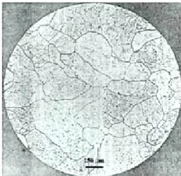
Figure 5. Microstructure of Delhi pillar iron (Published by Hadfield 13 ).
