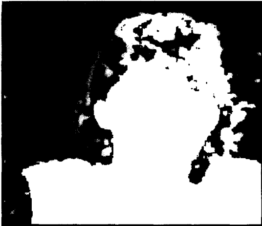
Fig. 5. Change mask obtained from Fig. 3 using the test statistic \bar{\Delta}_i^2 , \alpha = 10^{-2} , t_s = 44.3 . Due to the higher \alpha , there occur numerous detection errors in the background.
