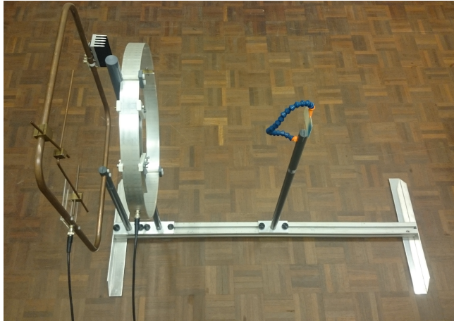
Fig. 9. Compact configuration of the antenna set-up, with activation and receiving antennas close together (on the left)
