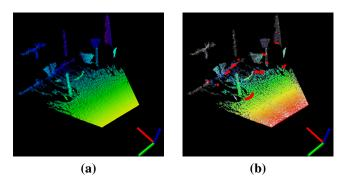
Fig. 2. Obstacle avoidance: The raw 3D point cloud (a) and (b) the sampled points (shown in color), along with the open path limits (red boxes). The robot location is marked by the axes.
