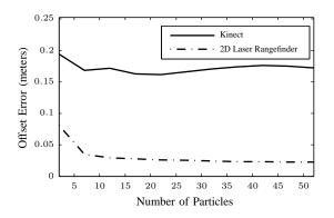
Fig. 3. The offset errors from the true robot locations while localizing using the Kinect *vs.* Laser Rangefinder
