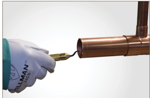
Figure 7.5. Reaming: Deburring Tool
