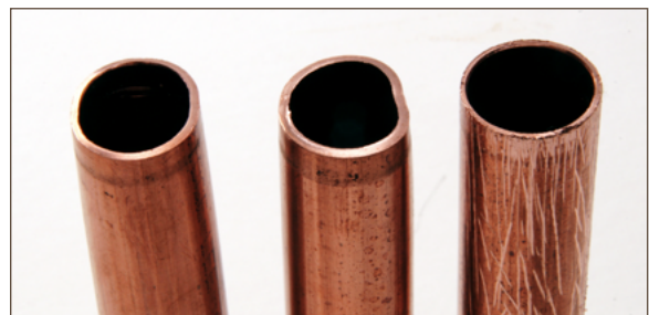
Figure 11.4. Inspect tube for imperfections
