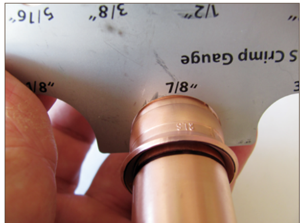
Figure 11.22. Correctly crimped fitting
