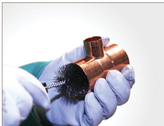
Figure 7.8. Cleaning: Fitting Brush
