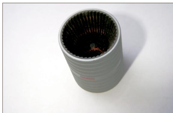
Figure 11.9. Combination tool for I.D. and burr removal
