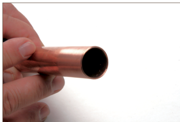
Figure 13.8. Reamed and deburred branch tube end
