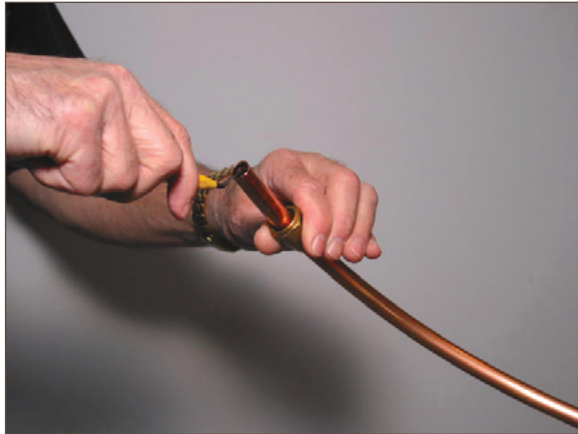
Figure 9.3. Reaming Prior to Flaring the Tube End
