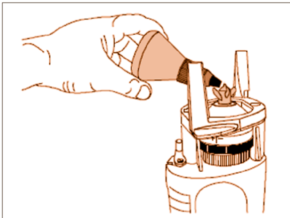
Figure 13.3: Lubricating the drill head
