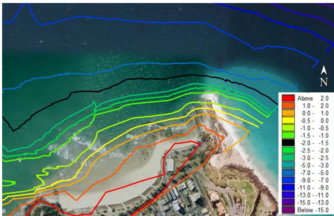
Figure 5 2D Contour map based on the interpolation of shore-normal hydrographic transect surveys taken on the southern Gold Coast
