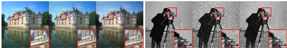
Figure 6: Qualitative results of image denoising tasks (BSD68 on the left, Set12 on the right). The noisy image is created with additive gaussian white noise ( \sigma = 50 ). We use an encoder embedding into \mathcal{W} of a StyleGAN 2 pre-trained on FFHQ.
