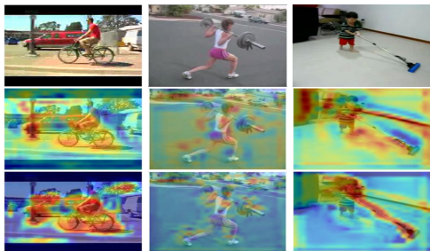
Figure 4: Visualization of feature maps on the UCF101 dataset. (From top to bottom) Input frames, output features of GCPN, and output features of GCPN convolved with filter kernels from LFMN. The bottom figures show higher response around the moving objects.
