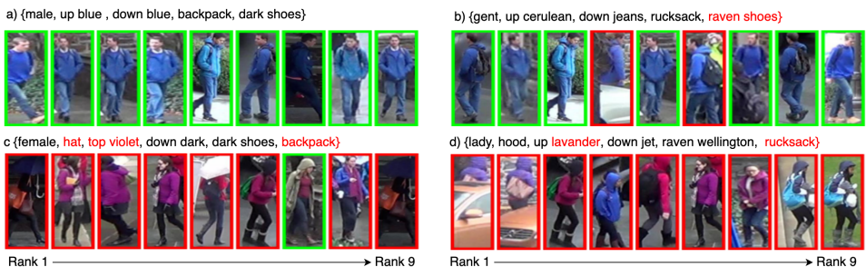
Figure 4: Text attribute queries in a),b),c) and d) and their top-9 ranked frame results. We indicate with green/red boxes the correct/false matches and highlight in red text the attributes that are not present in the retrieved frames.
