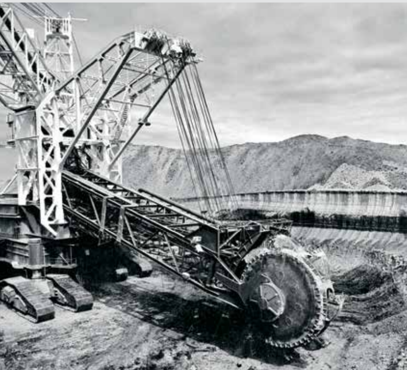
A distinctive feature in the early years at Glenharold Mine was the German-made Lauchenhammer wheel excavator, used only two years because the soil contained rocks too big for the machine to move.
