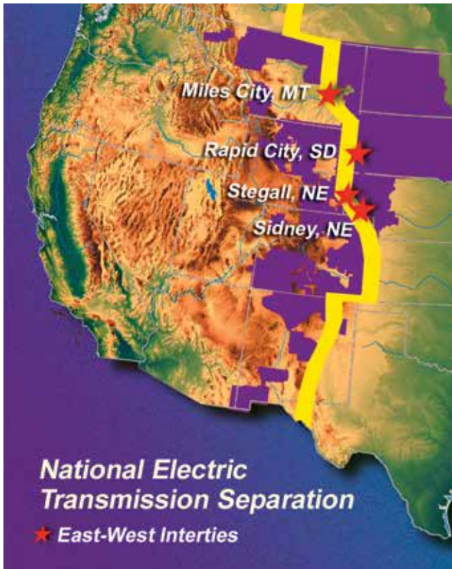
Basin Electric power resources and the membership service territories are located on both sides of the national electric transmission separation and cannot be connected directly except with a direct current (DC) tie. The tie takes alternating current (AC) from one side, converts it to DC, and then converts it back to AC.
