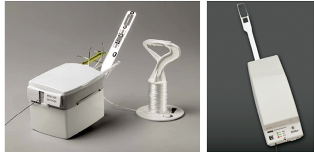
Figure 1. Picture of two radiosonde types used in this study: RS92 (left) and RS41 (right).
