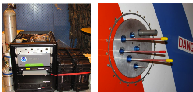
Fig. 2. NOAA equipment pallet for USCG C-130: three reference gas cylinders, instrument rack, and two Programmable Flask Packages (PFs) (left). Window replacement inlet plate (external view) (right).
