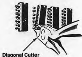
Figure 4-1 Removing IC (Cut-Pin Method)
