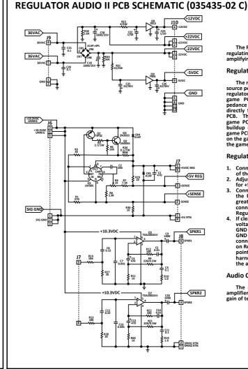
The Regulator/Audio PCB has the dual function of regulating the +5 VDC logic power to the game PCB and amplifying the audio from the game PCB.
