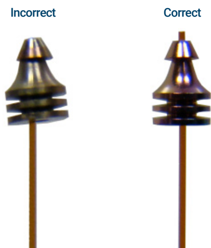
Figure 18. Incorrect and correct swaging symmetry
